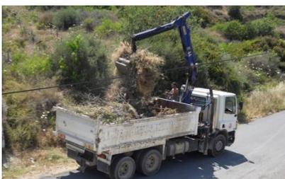
**Transport and loading:** Separate collection system for green waste with direct loading, or loading of on-site chipper prior to transport
